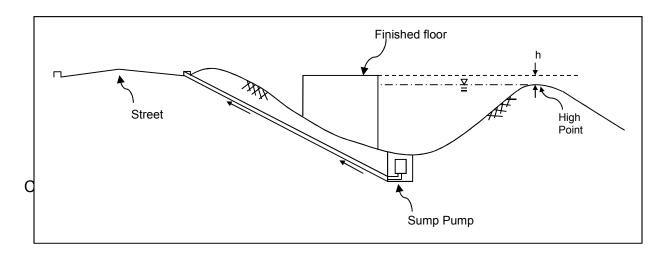
The finished floor elevation of the proposed project is below the sump overflow elevation, such as a condo complex with subterranean parking.
